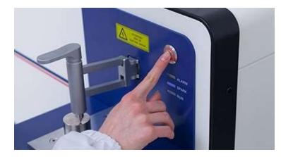
The ARTUS 8 uses a gas path protection device. If the instrument is not used for a long period of time, the gas path/light chamber purification time will not exceed 8 minutes.
